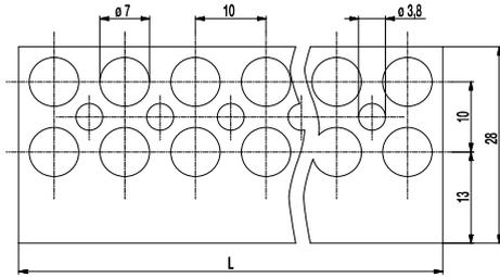
Marking strips BST-323 for our 323 series terminal strips are available in 2- to 12-pole and in 65-pole design (length: 650 mm). The customer can strip them easily to the desired pole number.
